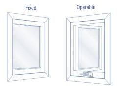
Among operable products, hinged windows (casement, awning, hopper, tilt, turn) are generally more airtight than sliding-style windows because the closing mechanism pulls them tight against the frame. Skylights should have a low curb (the part that holds the glass at the roof line) for better energy efficiency.
